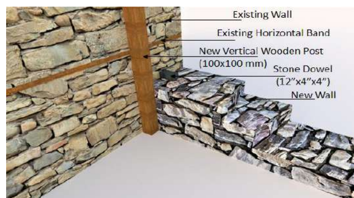
Figure 11. Stone dowels connecting the existing wall and the new wall in case of wooden reinforcement
