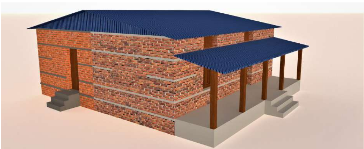
Figure 26. Addition of two rooms at one of the lengths with the provision of buttresses in case of brick in cement building
