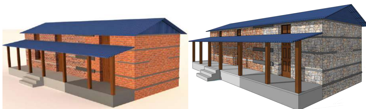
Figure 3. Addition of one room at one of the widths of the building
